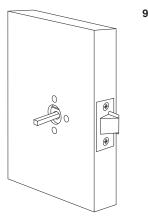
9. Pull off the rose covers. Remove the o-ring from the spindle, insert the spindle into the latch so an even amount protudes on each side of the door and slide the o-ring back onto the spindle.
