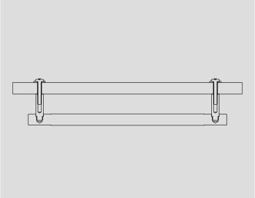
4. Ensure that you do not overtighten the screws.
