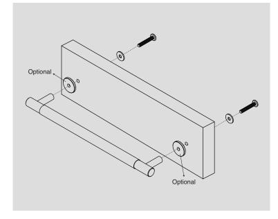
3. Hold the cabinet handle and align the legs with the pre-drilled 5.5mm diameter holes.
