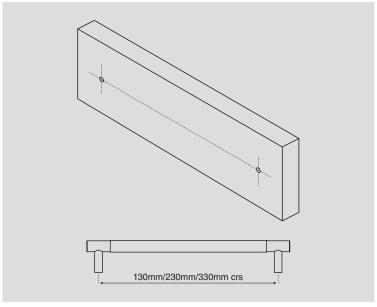
Drill two 5.5mm diameter holes at the marked fixing positions for the leg centres.
