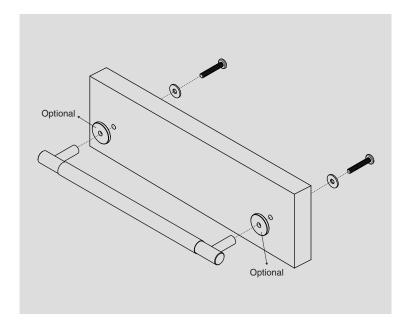
3. Hold the cabinet handle and align the legs with the pre-drilled 5.5mm diameter holes.
