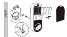
14. Connect the cable of the exterior unit to the interior unit. then align the interior unit and secure it with the screws. Insert 4 (AA)1.5V batteries and slide the battery cover onto the interior unit.
