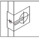
**3.** Establish the height and backset for the lock on the door.
