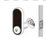
11. Install the touchpad deadbolt with the tailpiece in horizontal position inserted through the hub of the latch.
