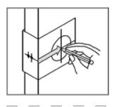
4. Use the template provided as an indication to mark the centre of the circle on the door face and the centre of the door edge.
