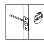
6. Insert the latch, scribe around the faceplate, remove, then chisel out 4mm deep recess to enable the latch faceplate to sit flush with the door edge.
