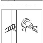
5. Use the marks as a guide for drilling a 25mm (1") diameter hole through the door edge to a depth of at least 90mm. Ensure this hole is square to the door. Then drill a 54mm diameter hole through the door face for the lockset. We recommend using a 54mm hole saw. For clean cut-outs, drill from both sides, meeting in the middle of the door.
