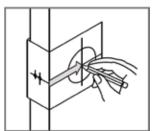
Use the template provided as an indication to mark the centre of the circle on the door face and the centre of the door edge.
