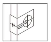
**3.** Establish the height and backset for the lock on the door.
