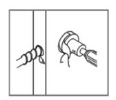
5. Use the marks as a guide for drilling a 25mm (1") diameter hole through the door edge to a depth of at least 90mm. Ensure this hole is square to the door. Then drill a 54mm diameter hole through the door face for the lockset. We recommend using a 54mm hole saw. For clean cut-outs, drill from both sides, meeting in the middle of the door.
