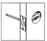
6. Insert the latch, scribe around the faceplate, remove, then chisel out 4mm deep recess to enable the latch faceplate to sit flush with the door edge.
