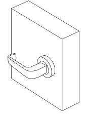
Screw the rose cover onto the handle and tighten the grubscrew on the side of the lever onto the spindle.
