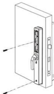
9. Insert 4 Alkaline (AA) 1.5V batteries\*, slide the battery cover onto the interior unit and tighten it with the screw provided.
