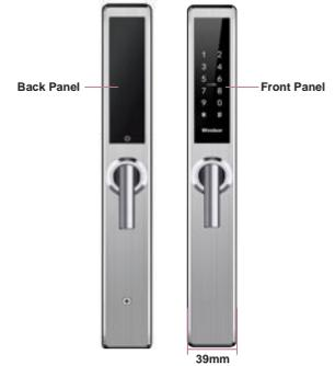
1. Ensure the lever is handed to suit your door. To adjust the handing, remove the Phillips screw in the back of the handle by turning it counterclockwise. Remove the lever and turn it around. Then insert the screw back into the handle seat and re-tighten by turning it clockwise\*. Both front and back panels will require this adjustment.
