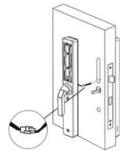
8. Hold the front panel against the door face, sliding the spindle and threaded sleeves through the drilled holes. Install the back panel by tightening the screws through the back panel into the threaded sleeves. Ensure the panels are sitting straight on the door.
