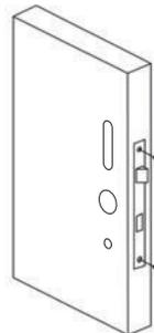
3. Install the spindle into the back of the lever of the front panel. Insert the split pin and bend its front end to fix it into the square shaft (b). Turn the spindle and square shaft to ensure the small arrow is pointing towards the hinges (a).
