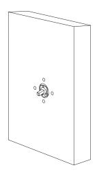
Fit the dummy spindle by drilling and fitting the three wood screws provided. Ensure the grooved side of the spindle will align with the grubscrew on the handle.
