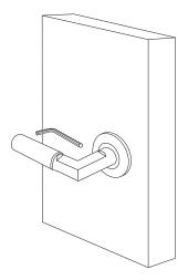
Screw the rose cover onto the handle and tighten the grubscrew on the side of the lever onto the spindle.
