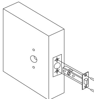
4. Insert the latch, scribe around the faceplate, remove, then chisel out recess to enable the latch faceplate to sit flush with the door edge.
