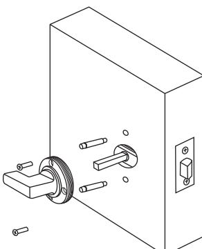
6. Unscrew the rose covers from the turns and unscrew the bolts from the threaded sleeves.
