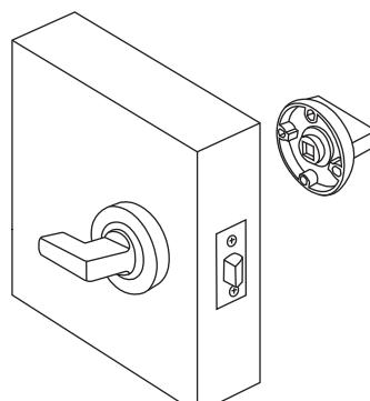
10. Insert the other turn on the opposite side of the door over the spindle and tighten the long bolts through the rose into the threaded sleeves.
