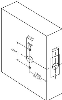
1. Measure the door thickness and mark the centre at the desired height for the bolt.
