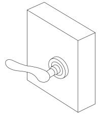
**6.** Screw the rose cover onto the handle and tighten the grubscrew on the side of the lever onto the spindle.
