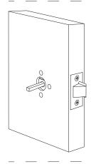
9. Pull off the rose covers. Remove the o-ring from the spindle, insert the spindle into the latch so an even amount protudes on each side of the door and slide the o-ring back onto the spindle.
