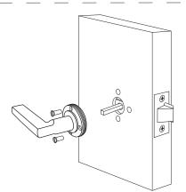
10. Insert the blind nuts through the face of the rose at two vertical positions. Slide the handle over the spindle and press against the door.
