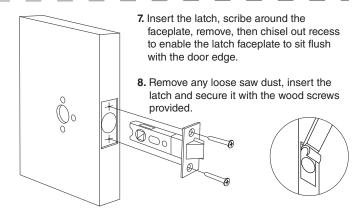
Note: To change the handing of the latch, pull out the tongue and then twist to rotate the position of the tongue.
