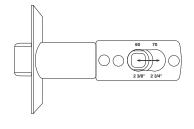
1. Change the position of the latch to 60mm or 70mm backset by sliding the latch body back and forth.
