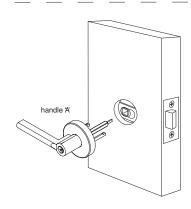
7. Insert handle 'A' wth the spindle attached in the 54mm hole through the latch and press against the door.
