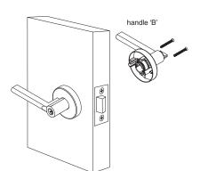
8. Insert 'handle B' on the opposite side of the door over the spindle. Align the latch guide prongs and ensure the handles are straight before securing the through fixing screws.
