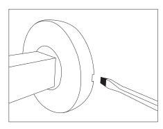
To remove the rose cover off the handle, use a flat head screwdriver, ideally the same width as the groove on the side of the rose.
