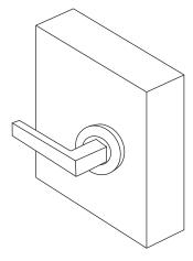
6. Press the rose cover onto the handle and align the dimples on the sides of the rose. Tighten the grubscrews on the side of the lever onto the spindle.
