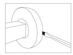
2. Insert the screwdriver into the groove on the side of the rose.
