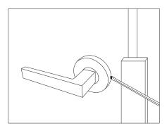
3. To protect the door from getting damaged, use a small wooden block or something similar and use the screwdriver as a lever.
