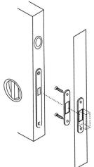
7. To fit the keeper, slide the door into closed position and transfer the lock markings to the door jamb. Mark the centre of the lock bolt in retracted position. Centre up the keeper hole with the centre of the bolt. Screw the keeper plate to the door jamb and scribe around the outside. Mark the centre hole for the mortice, remove the plate and mortice the centre hole to a depth of 20mm. Chisel out a 2mm recess to accept the keeper plate.
