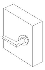
6. Screw the rose cover onto the handle and tighten the grubscrew on the side of the lever onto the spindle. For the square rose (Astron Elite) press on the rose cover and tighten the grubscrew on the side of the rose.
