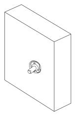
Fit the dummy spindle by drilling and fitting the three wood screws provided.
