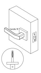
8. Insert the spindle into the latch and into handle A. Ensure the grooved side of the spindle will align with the grubscrews on the handles. Slide handle B' over the spindle onto the mounting plate, press against the door and tighten the grubscrew on the side of the rose to the mounting plate.
