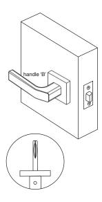
5. Insert the spindle into the spindle hole and into handle 'A'. Ensure the grooved side of the spindle will align with the grubscrews on the handles. Slide handle 'B' over the spindle onto the mounting plate, press against the door and tighten the grubscrew on the side of the rose to the mounting plate. Tighten the grubscrews on the side of the levers onto the
