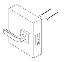
4. Slide the handle onto the spindle ensuring that it sits straight on the door face. Fix the two through bolts provided from the opposite side of the door into the handle. Trim the bolts to the correct length if necessary. Tighten the grubscrew on the side of the lever onto the spindle.
