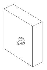
3. Fit the dummy spindle by drilling and fitting the three wood screws provided. Ensure the grooved side of the spindle is aligned with the grubscrew on the handle.
