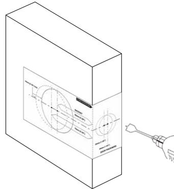
2. Fold the template where indicated on the door edge at the desired deadbolt height. Firmly hold the template in place.
