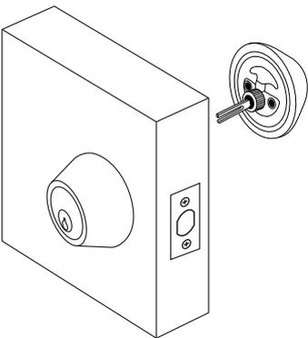
8. Press the internal cylinder/turn flush against the opposite side of the door, ensuring the keyhole/turn is pointing down. For the cylinder ensure the spindle is being inserted through the deadbolt vertically. For the turn the slot for the spindle will be in horizontal position to be able to fit the spindle of the external cylinder. Fasten the cylinder/turn with the screws provided.
