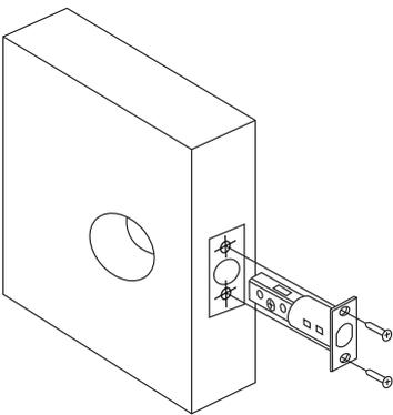
5. Insert the deadbolt, scribe around the faceplate, remove, then chisel out a 4mm recess to enable the faceplate to sit flush with the door edge.
