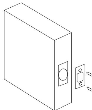
9. Close the door against the door frame with the deadbolt extended and mark the deadbolt position for fitting of the striker.
