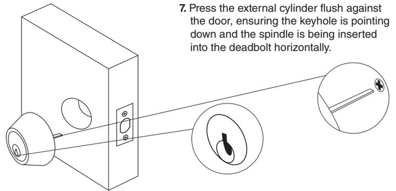
7. Press the external cylinder flush against the door, ensuring the keyhole is pointing down and the spindle is being inserted into the deadbolt horizontally.
