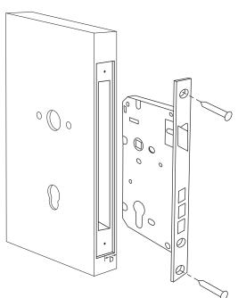
7. Check the latch tongue is facing the correct way to latch on the door frame, reverse if necessary by lifting up the tab behind the latch tongue, push the latch tongue into the lock case and rotate 180 degrees, then release the latch tongue and ensure the tab is returned to the downward position.
