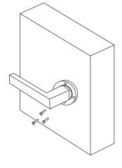
Install the handle by screwing the base plate to the door with the wood screws provided.
