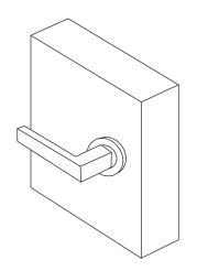
Screw the rose cover onto the handle and tighten the grubscrew on the side of the lever onto the spindle. For the square rose (Futura Elite) press on the rose cover and tighten the grubscrew on the side of the rose.
