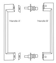
Take the pull handle apart by unscrewing the grubscrews on both legs and then unscrewing the bolts with a 5mm allen key.
