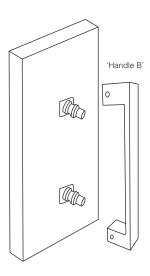
Insert 'Handle B' onto the brass mounts and secure it with the grubscrews.
