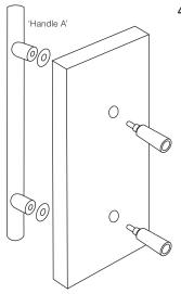
Insert the bolts through the legs and then through the door and tighten them onto 'Handle A'.
