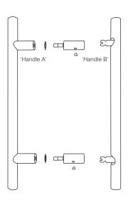
Take the pull handle apart by unscrewing the grubscrews on both legs and then unscrewing the legs.
