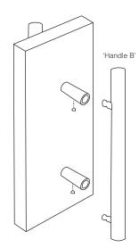
5. Insert 'handle B' into the pull handle legs and secure it with the grubscrews.
